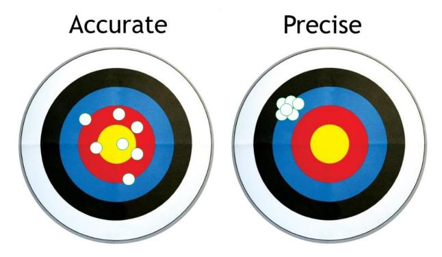
Figure 4 | Accuracy versus precision
