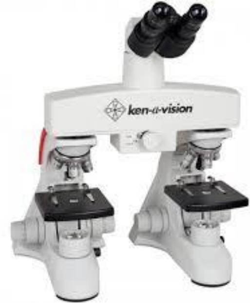
Comparison microscope with 2 stages to compare evidentiary samples side-by-side
